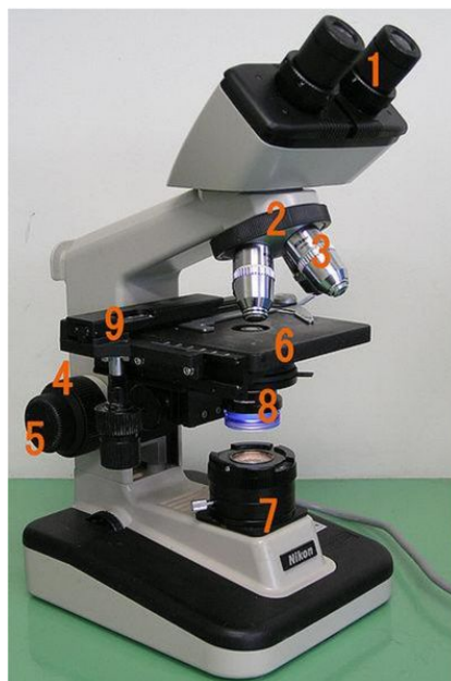
Rysunek 1: Construction and working principle of bright field microscope: 1. ocular lens; 2. revolver (to hold multiple objective lenses); 3. objective lenses; 4. focus knob - coarse adjustment; 5. focus knob - fine adjustment; 6. stage; 7. light source; 8. condenser; 9. mechanical stage
