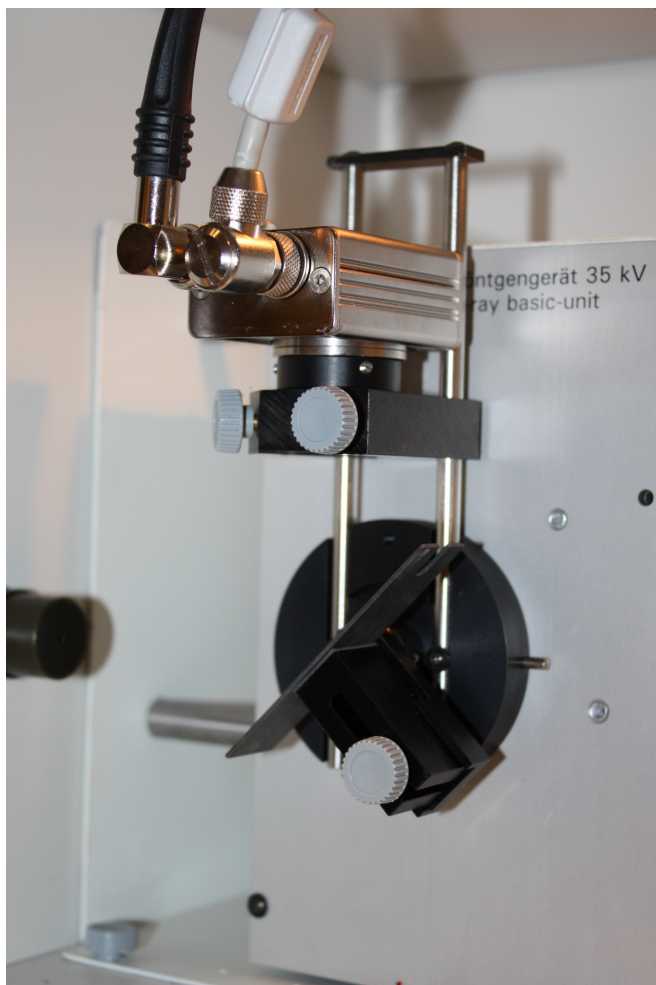
Fig. 4: Fitting the X-ray energy detector to the goniometer.
